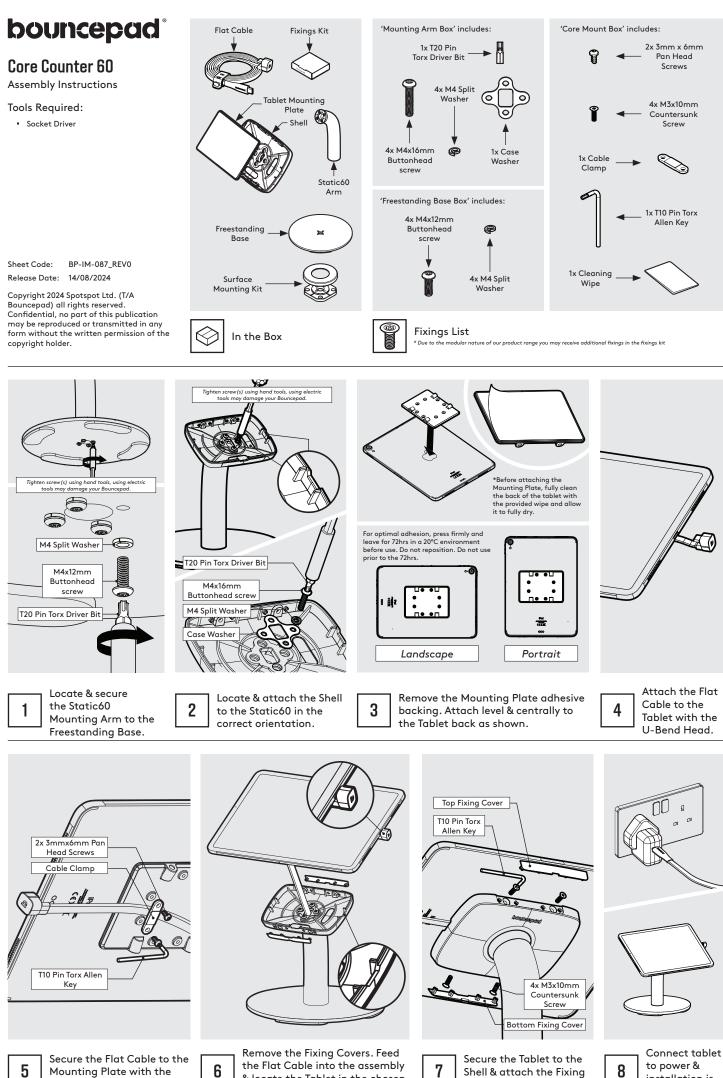
Mounting Plate with the Cable Clamp as shown.
