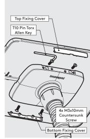
Secure the Tablet to the Shell & attach the Fixing Covers as shown.
